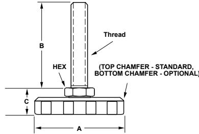
Optional bottom chamfer (reverse assembly) – with 90° top edge
