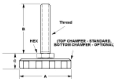
Optional bottom chamfer (reverse assembly) – with 90° top edge
